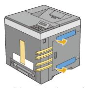
Pull the protective sheet out of the printer.
